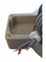
Strip about 10mm of both ends. Remove the shield on the shorter end.
