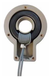
Put a winding with 8 turns on the core as shown.
